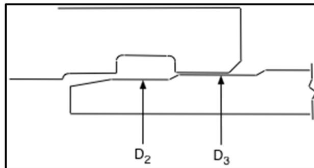
Figure B.1: Coupling and Spigot End of AC Pipe
