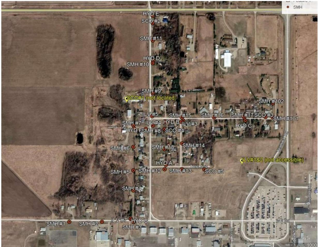
Figure 5.2: Location of Inline Valves and Hydrants
