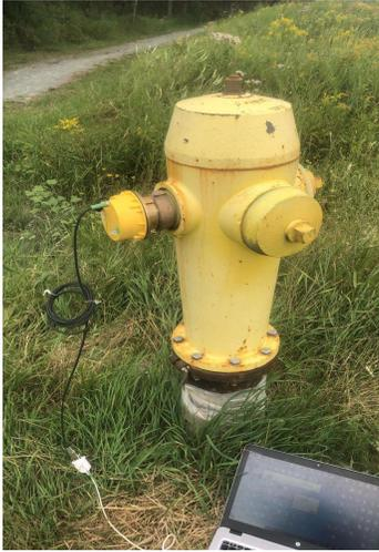
Figure 4.3: Telog HPR on Hydrant
