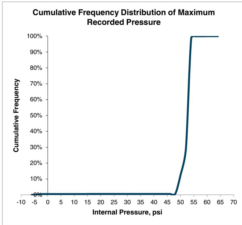
Figure 6.3: Cumulative Frequency Distribution of Maximum Pressure
