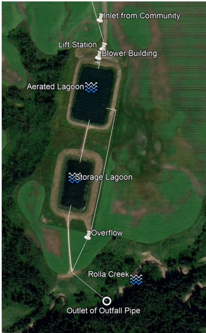
Figure 2 - Wastewater Treatment Plant - Layout
