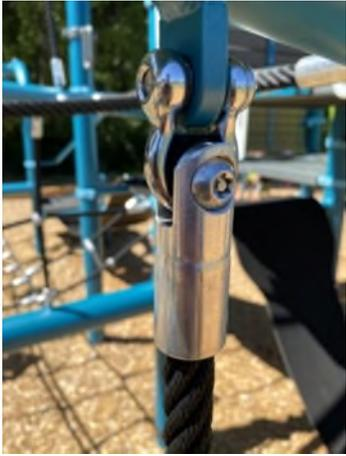
**Aluminum Net Connectors:** All climbing net connections are made with metal parts that stand the test of time. Beware of plastic connectors that break down in UV light and the dynamic stresses created by flexible cable. For longevity, all dynamic cable play should connect to the structural framework via a flexible connection. This prevents the cable from “paper clip” fracturing.
