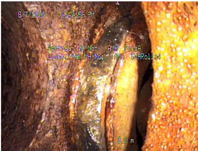
Figure 12 - Severe Corrosion in Valve Between Lagoons
